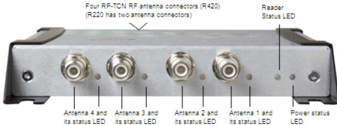
Figure 5.2 Speedway Revolution R420 Antenna Ports and Status LEDs
